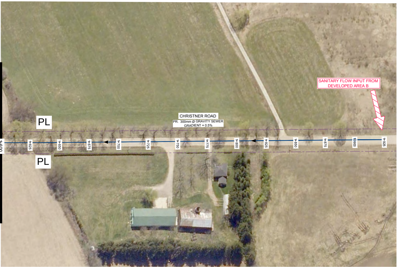
ALTERNATIVE C - PROPOSED SEWER ALIGNMENT PROFILE
