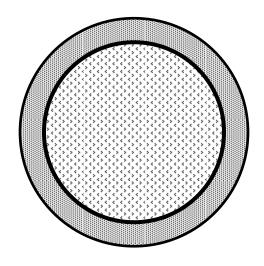
A circle of stones or a cement ring style of burn pit may be used. The area around the circle of approximately 25cm or 10 inches (indicated by the dotted area in the diagram) should be clear of dry or dead grass or other combustible materials that may be ignited by heat radiated through the stones or cement. The size of the circle should be the approximate size of a tire rim. (About 60cm (24 inches) in diameter).
